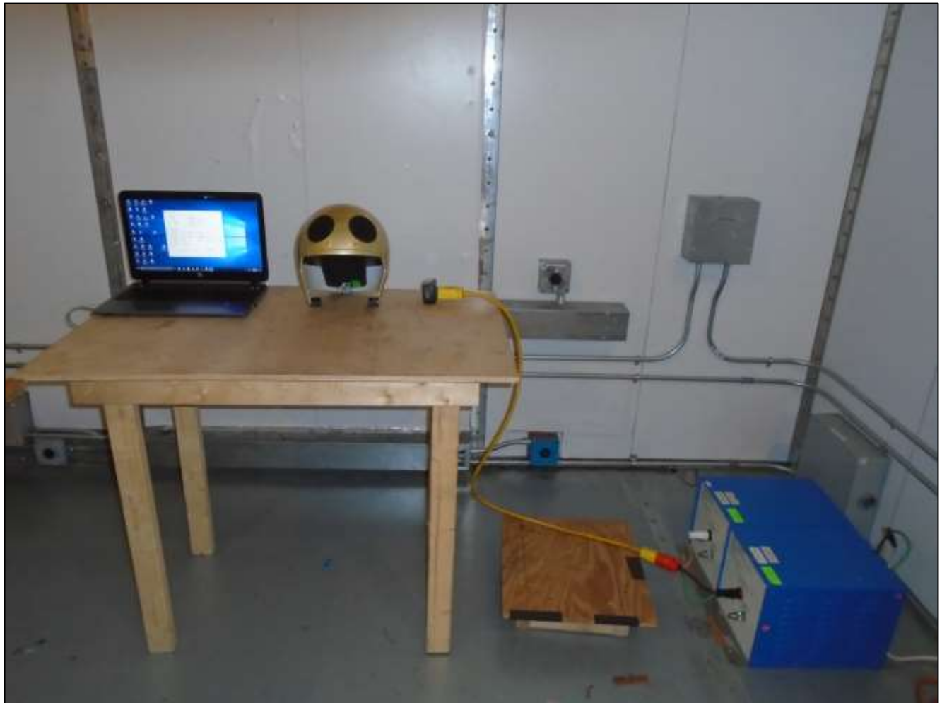
Photograph 1. Conducted Emissions, 15.207(a), Test Setup
