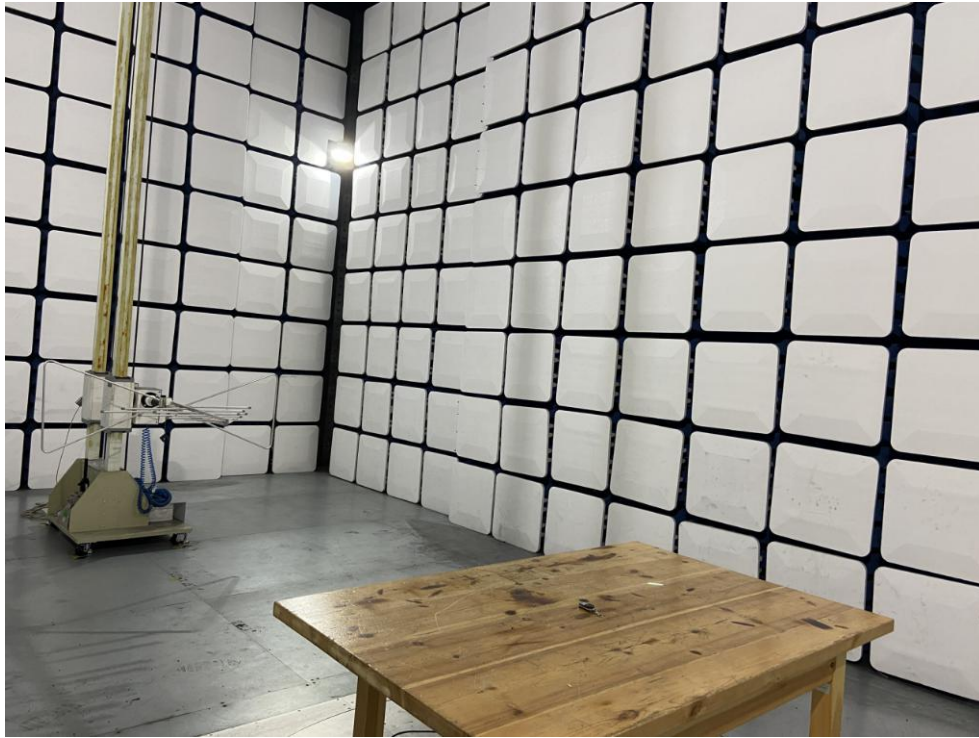
FCC ID: 2APKA-WCR100 Photo of Radiation Emission Test
