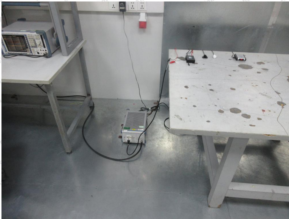
Photo of Radiated Emission Measurement
