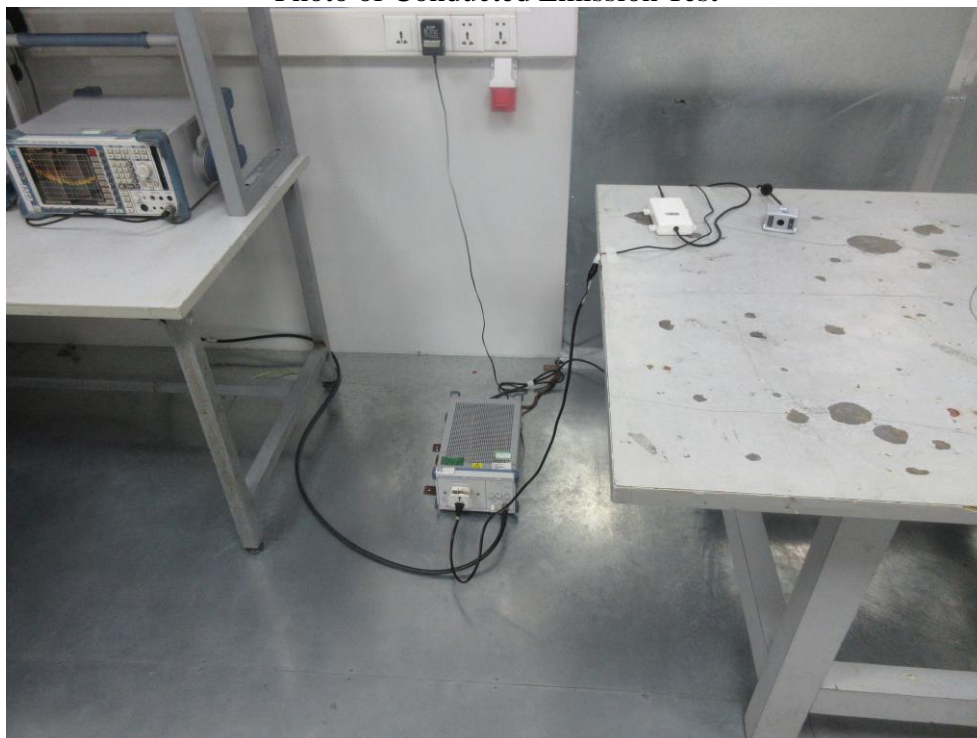
Photo of Radiation Emission Test
