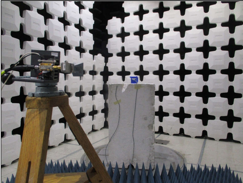
Test Setup for Spurious Radiated Emissions, 18GHz to 25GHz – Antenna Polarization Horizontal
