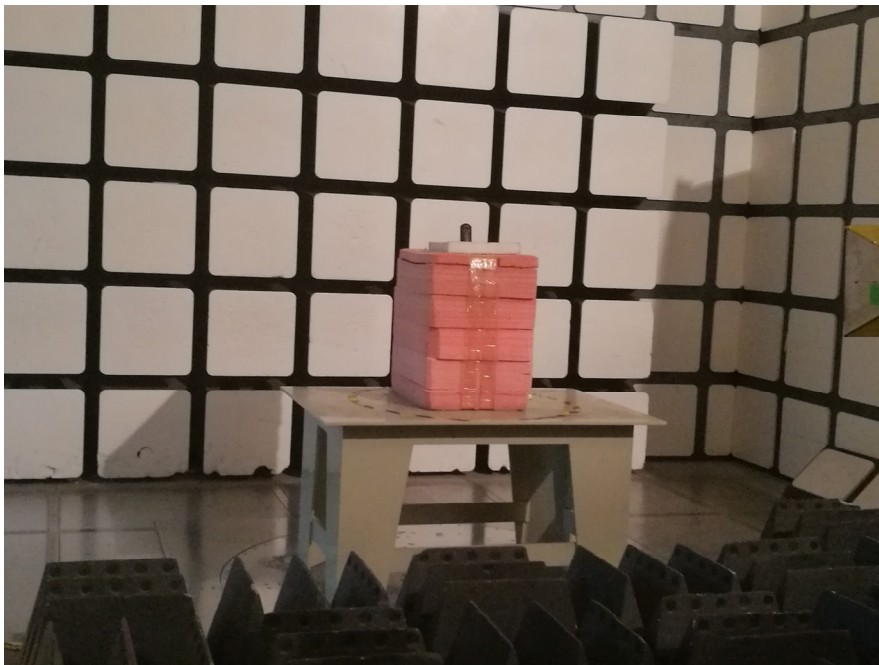
Radiated Emissions View (Above 1 GHz)
