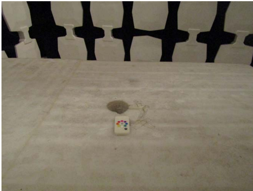
Measurement of Radiated Emission Test Set Up
