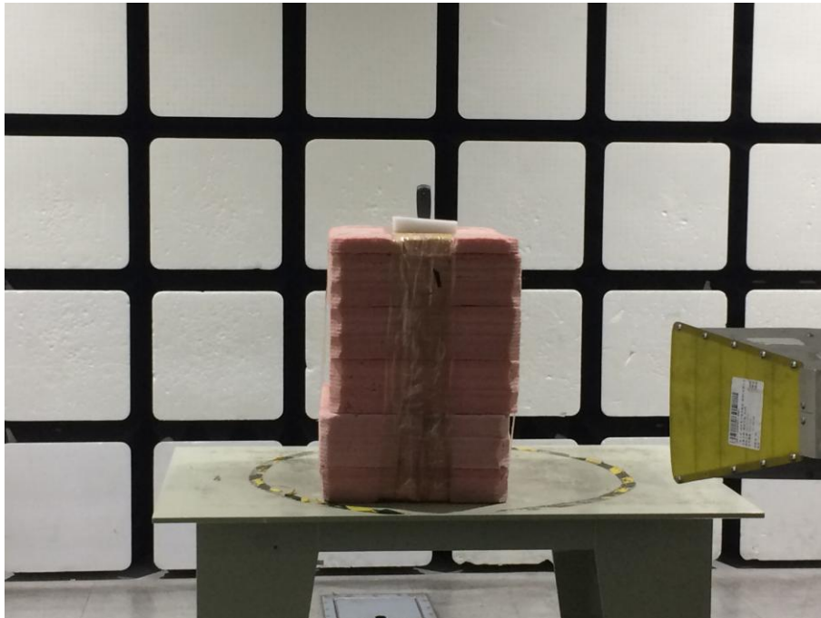
Radiated Emissions View (Above 1 GHz)
