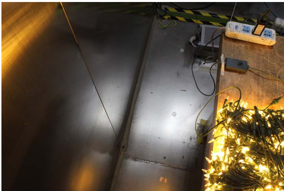
Conducted Emissions - Side View
