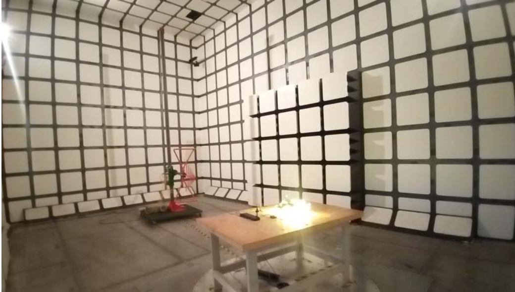
Radiated Emissions View (Below 1 GHz)
