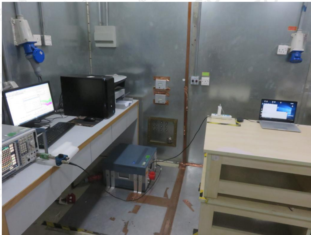
FCC RADIATED EMISSION TEST SETUP
