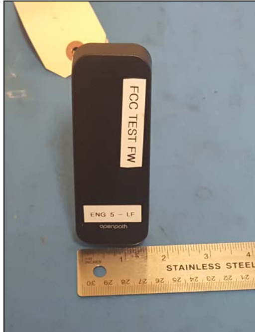
Photograph 1. Openpath Security Inc. Smart Reader & Mullion Smart Reader (LF) with Taiyo Yuden Model EYSGJN
