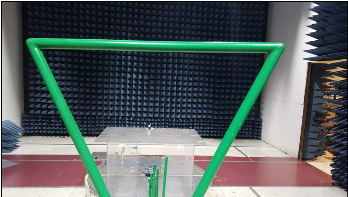
Photograph 2. Radiated Spurious Emissions, Test Setup, 30 MHz – 1 GHz
