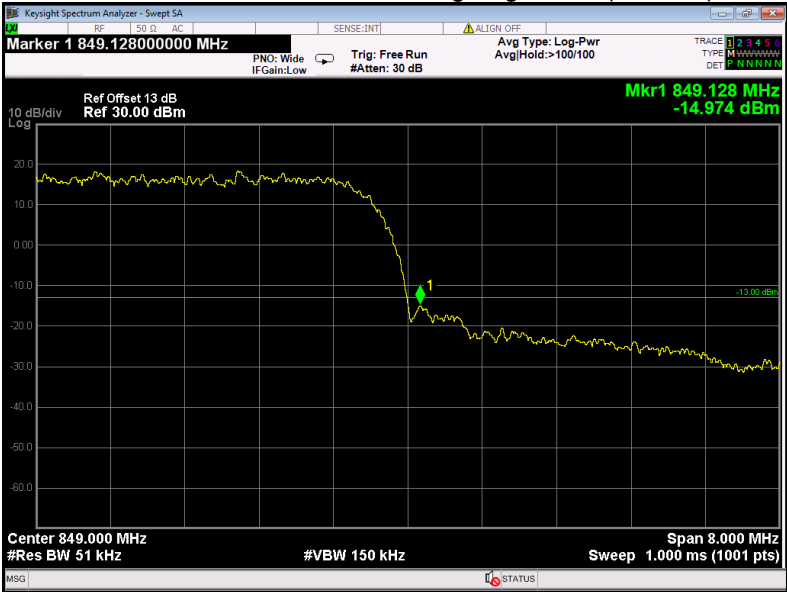
WCDMA band V band edge-right side (HSUPA)
