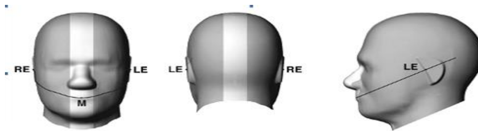
F-3. Front, back, and side views of SAM (model for the phantom shell). Full-head model is for illustration purposes only-procedures in this recommended practice are intended primarily for the phantom setup.
