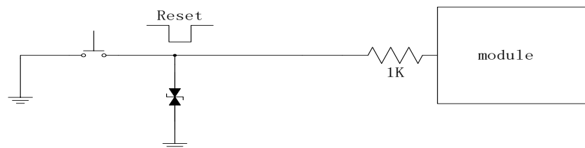
Figure 4.7: Reference design of key reset circuit
