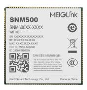
SNM500 adopts Qualcomm QCM2150 platform, 4-core A53(4\* 1.3GHz) with 28nm FinFET process, 64bit ARM. It supports decode/encode up to 1080P@30fps, H.264, HD+ screen resolution, and dual ISP cameras. SNM500 is equipped with Android 10 operating system and a board memory of 1GB+8GB (2GB+16GB, and 3GB+32GB).
