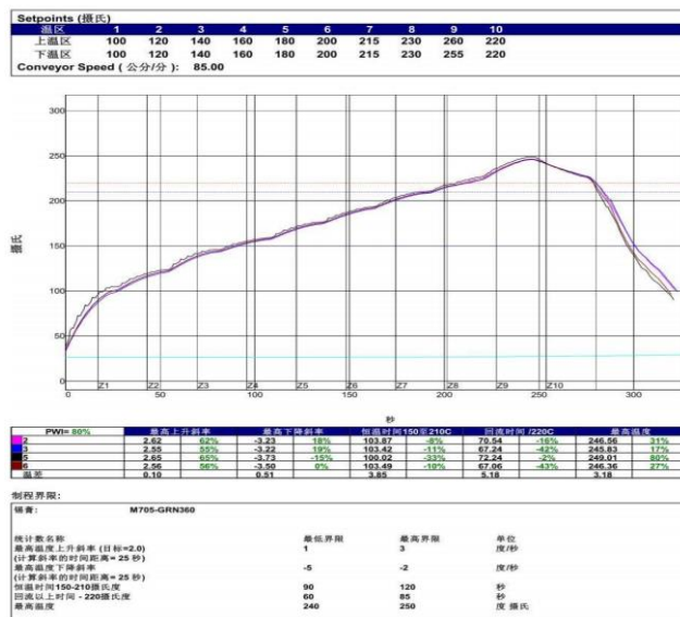
Figure 32 Temperature curve of solder reflow
