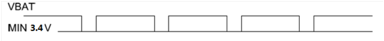
Figure 4.4: VBAT lowest voltage drop
