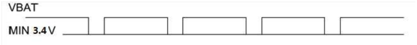
Figure 4.4 : VBAT lowest voltage drop
