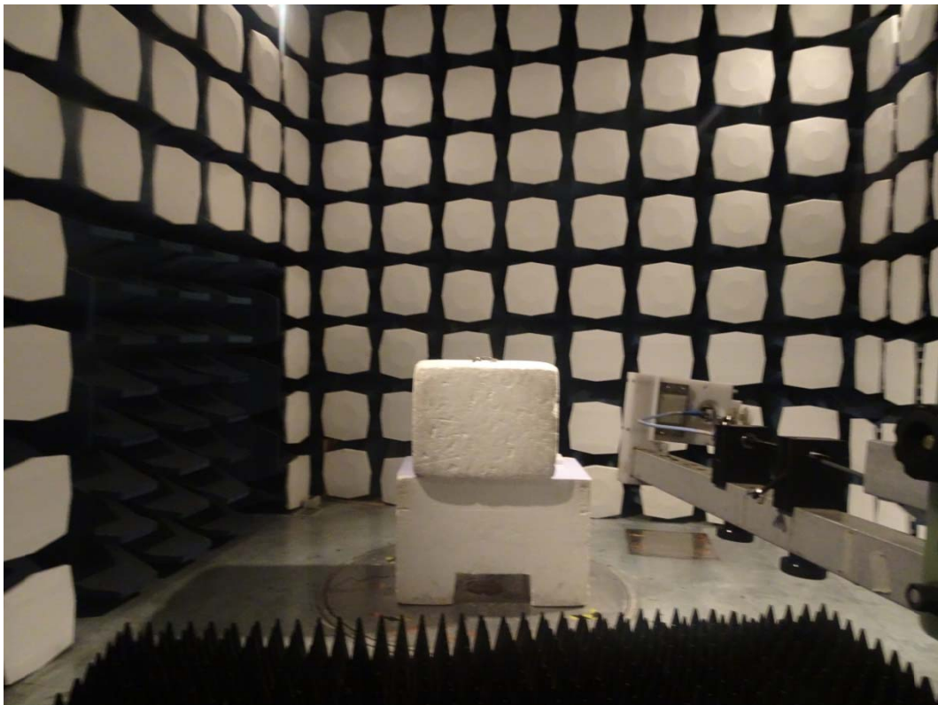
Picture 1: Radiated Spurious Emissions Test setup
