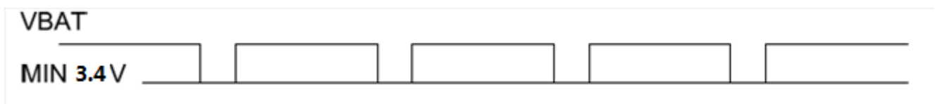
Figure 11 VBAT lowest voltage drop
