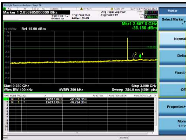
GFSK LOW CHANNEL, SPURIOUS 30 MHz ~ 3 GHz
