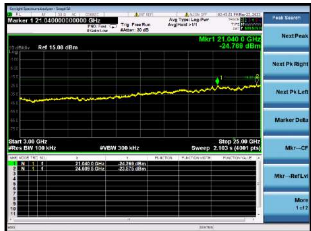
GFSK LOW CHANNEL, SPURIOUS 3 GHz ~ 25 GHz
