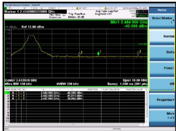
GFSK HIGH CHANNEL, BAND EDGE
