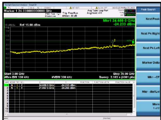
GFSK HIGH CHANNEL, SPURIOUS 3 GHz ~ 25 GHz
