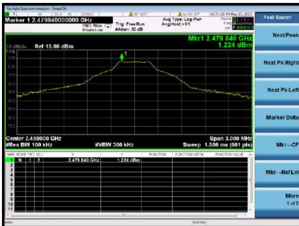
GFSK HIGH CHANNEL, CARRIER LEVEL
