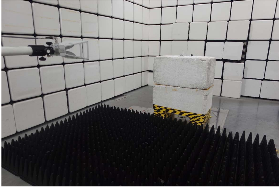
Picture 1: Radiated Spurious Emissions Test setup
