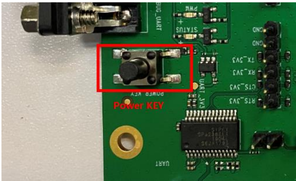
Figure 12 Power-on key location diagram
