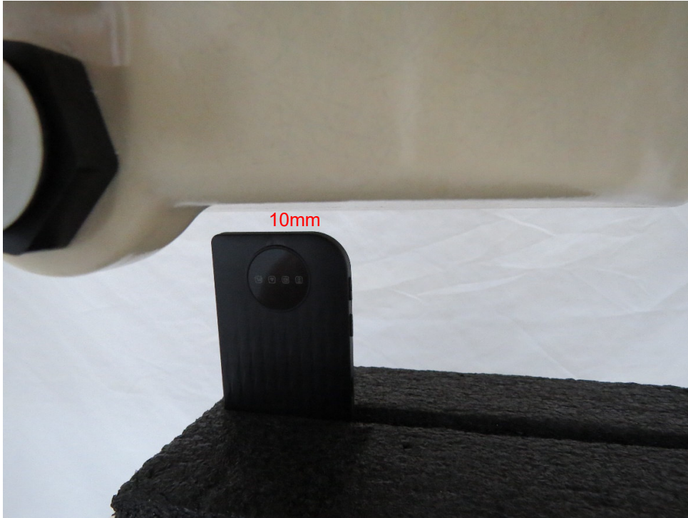
Picture 5: Top Edge, the distance from EUT to the bottom of the Phantom is 10mm
