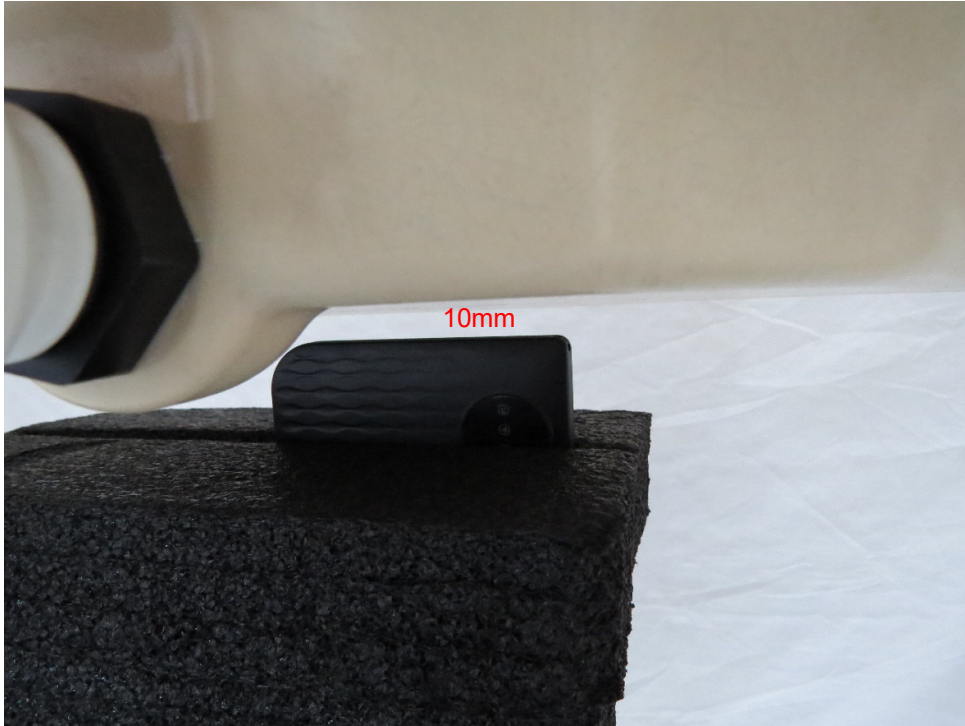
Picture 3: Left Edge, the distance from EUT to the bottom of the Phantom is 10mm
