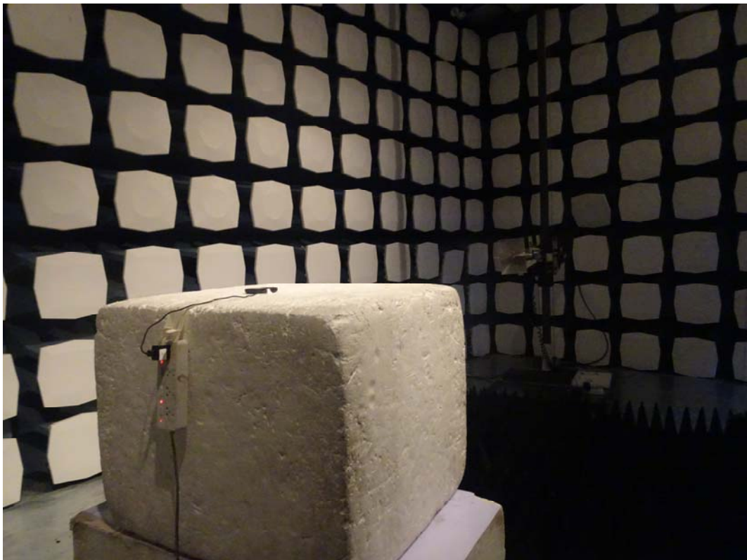
Picture 1: Radiated Spurious Emissions Test setup
