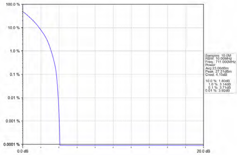
n12_15kHz_SISO_NTNV_10MHz_DFT-s-OFDM PI/2 BPSK_711MHz_Outer_Full
