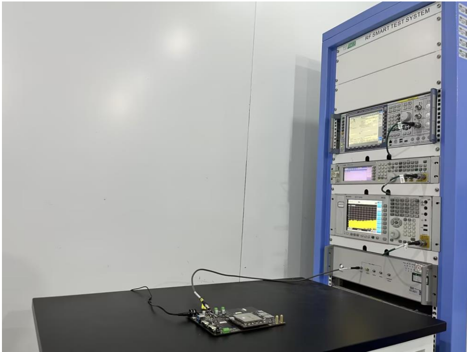
RF conducted test setup
