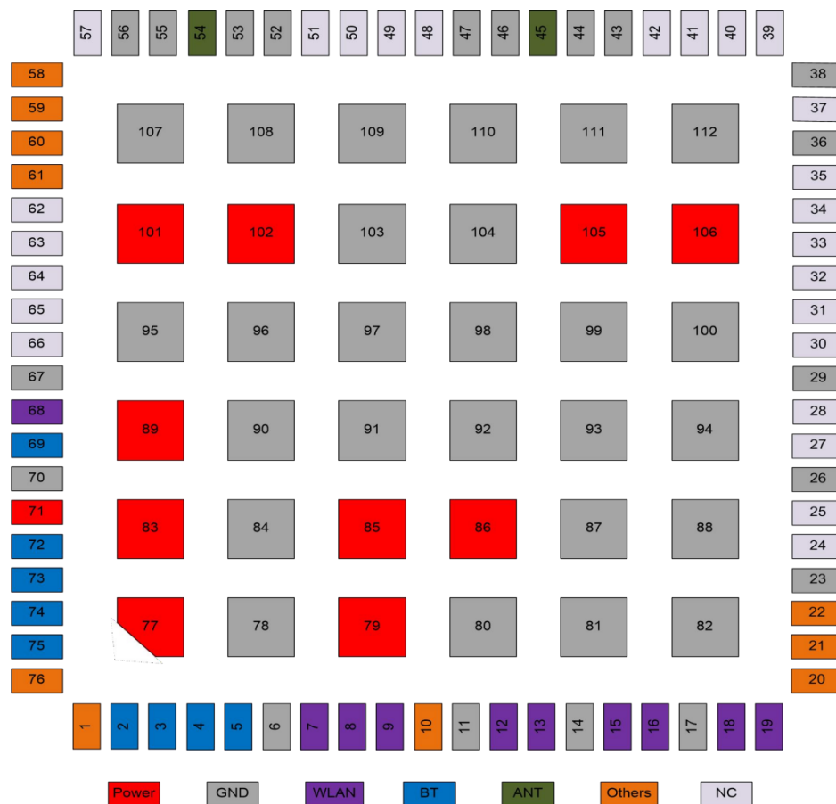
Figure 2: MA188 Pin Assignments(top view)
