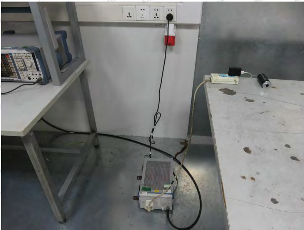
Photo of Conducted Emission Measurement
