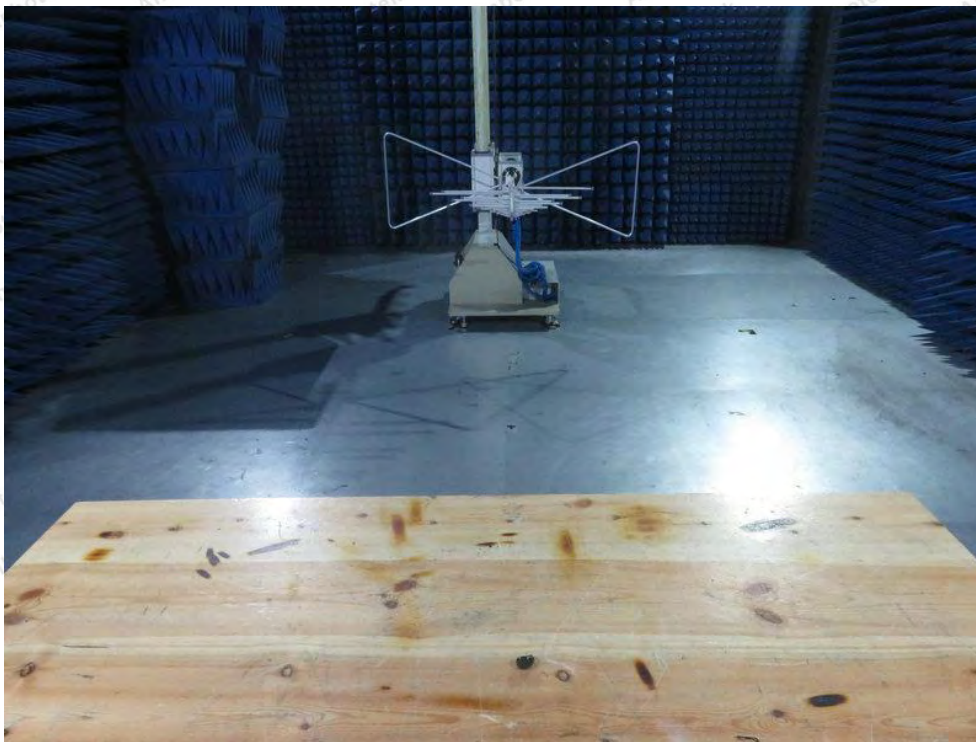
Photo of Radiation Emission Test
