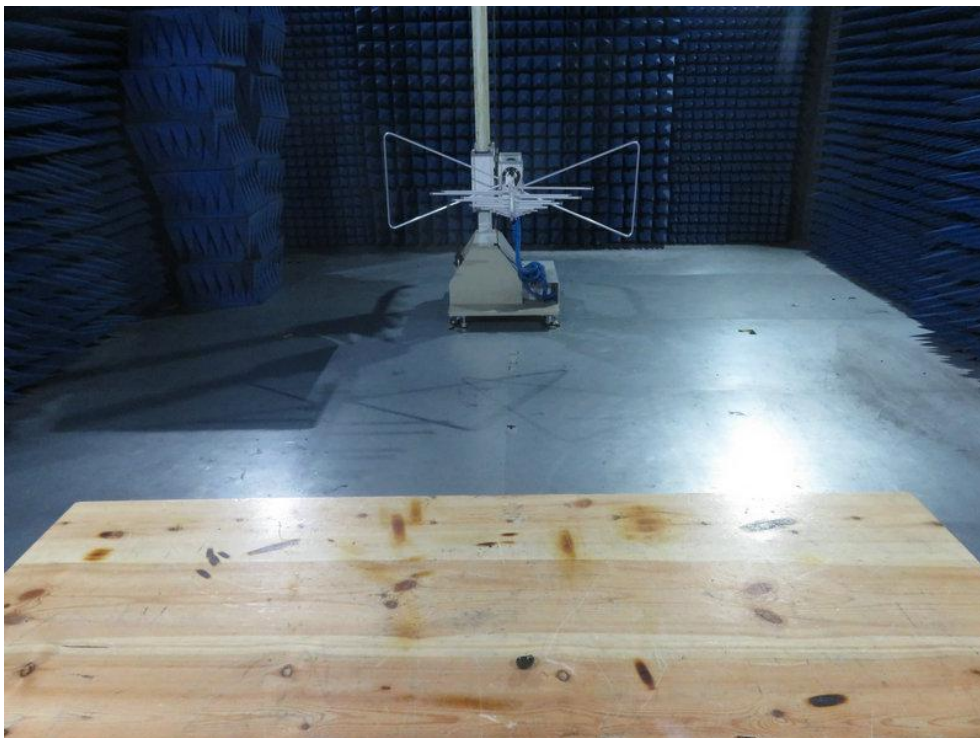
Photo of Radiation Emission Test
