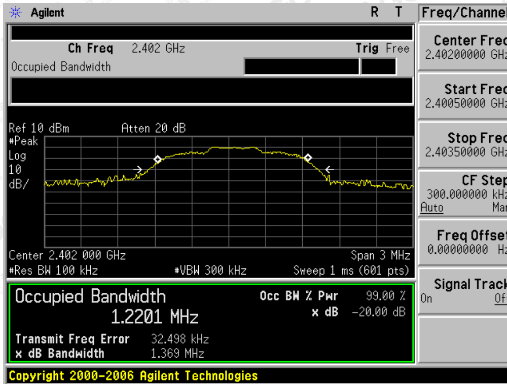
TEST PLOT OF BANDWIDTH FOR LOW CHANNEL
