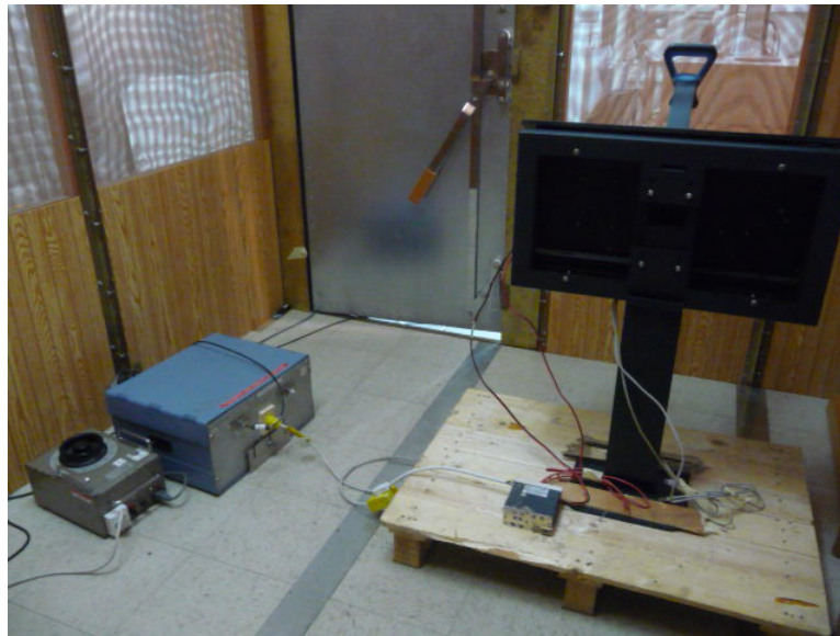
Photograph 8.1.1 Setup for conducted emission measurements
