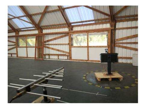
Photograph No.4 Radiated emissions measurement setup at the OATS in 200 – 1000 MHz
