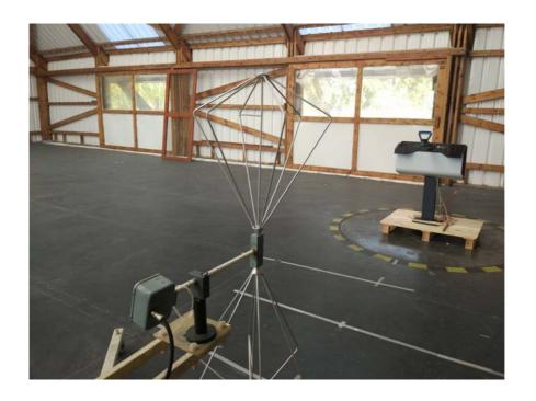
Photograph No.3 Radiated emissions measurement setup at the OATS in 30 – 200 MHz
