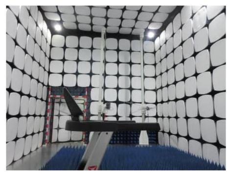
Remark: The transmitter part of the EUT was kept on the high 0.8 m below 1 GHz and 1.5 m above 1 GHz according to the lifting platform during the test.
