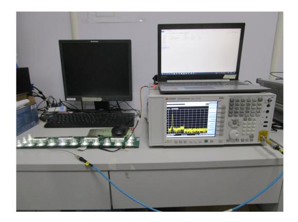
1.3 Radiated Emissions which fall in the restricted bands & Radiated Spurious Emissions Test Setup
