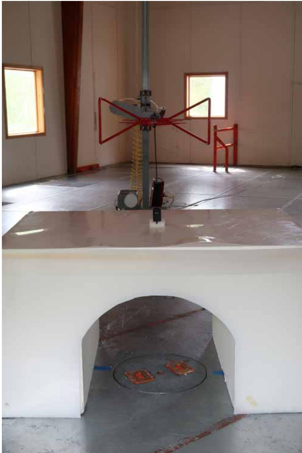
**8. Test Setup Photographs****8.4. Radiated Emissions above 1 GHz – Front**
