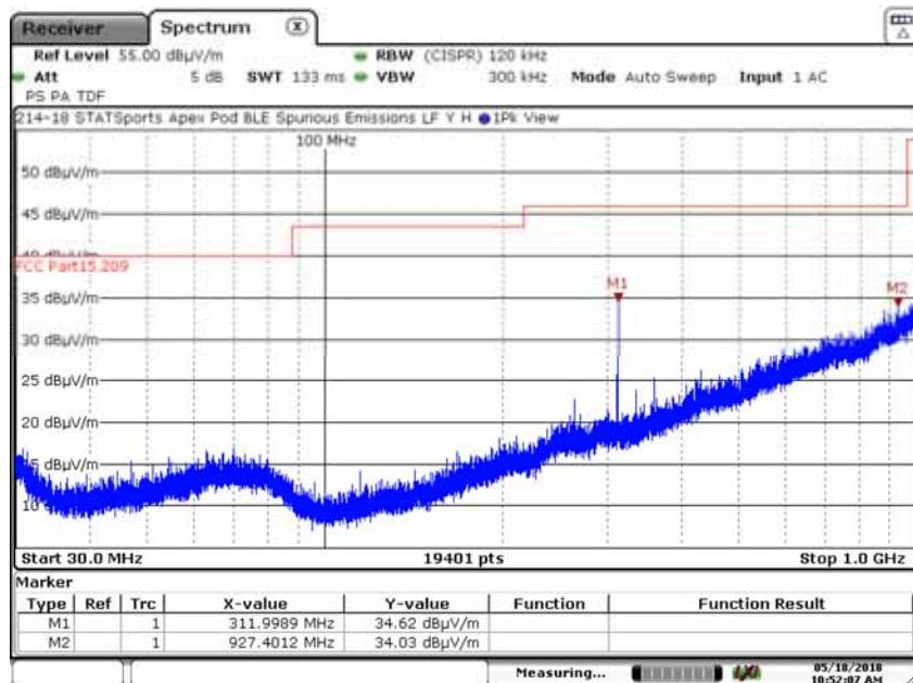
**A3.1.4. Measurement Results: Y-Axis, Vertical Antenna**
