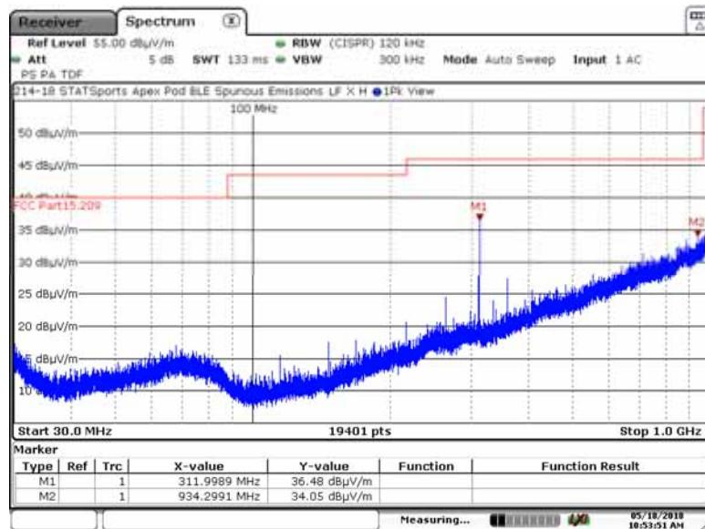
**A3.1.2. Measurement Results: X-Axis, Vertical Antenna**
