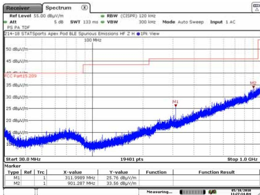
**A3.3.6. Measurement Results: Z-Axis, Vertical Antenna**
