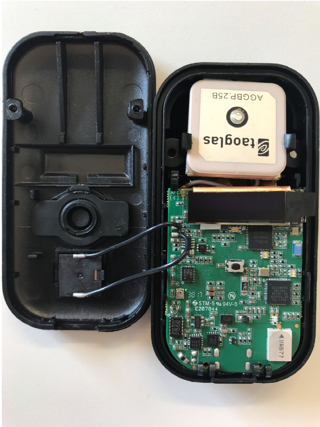
APEX PCB (FRONT) Fitted in Casing
