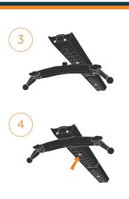
Second: Connect the legs to the bottom of the tracks by inserting them into the magnetic ports on the bottom of the track. Attach them to whichever port will satisfy the terrain you want to shoot on. (You can also attach a tripod to the bottom of the track via the threaded inserts as indicated by the orange arrow).
