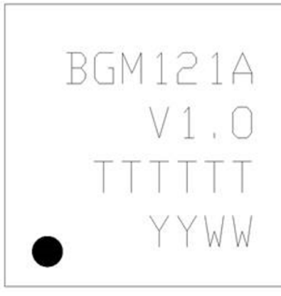
Figure 8.4. BGM121/BGM123 Package Marking
