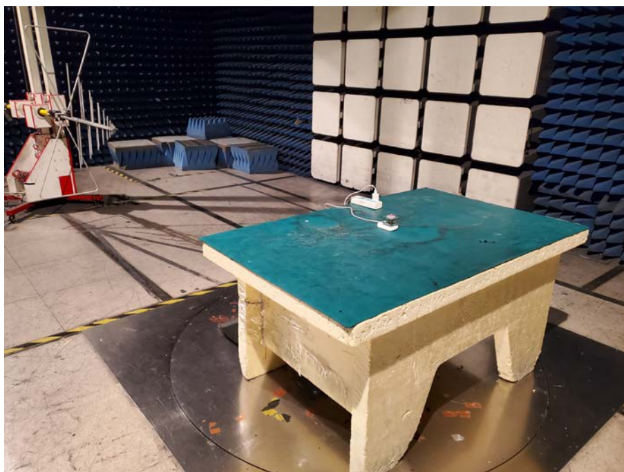
Spurious Emission Test Setup (Below 1GHz)
