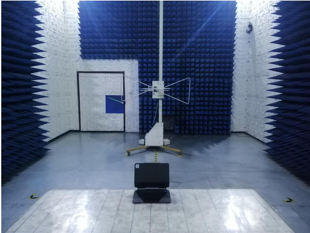
RADIATED EMISSION TEST SETUP ABOVE 1GHz
