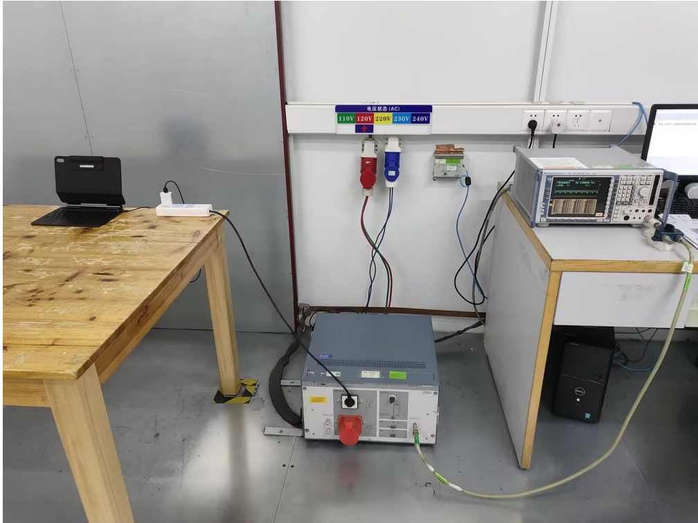
The series model: 6B016A RADIATED EMISSION TEST SETUP BELOW 1GHz
