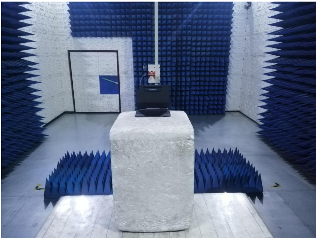
RADIATED EMISSION TEST SETUP ABOVE 1GHz
