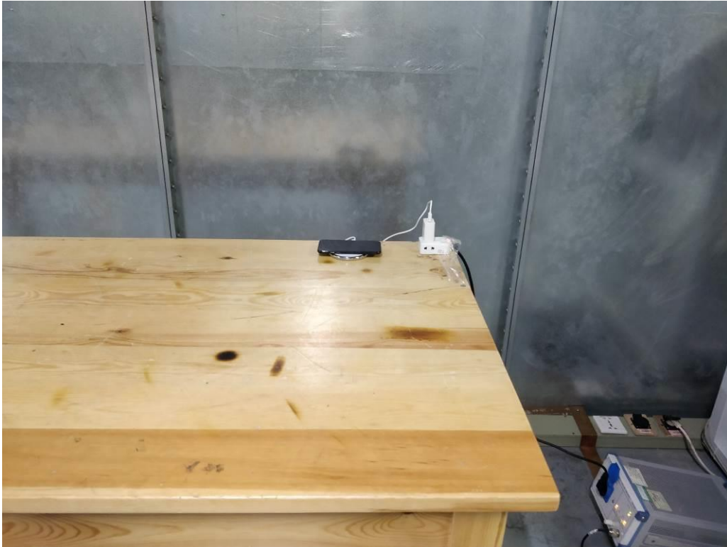
Conducted Emission-AC adapter charge mode
