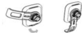
Turn the Cradle downwards to USB Port to lock it up. When not needed, you can put the support aside, or detach it.
