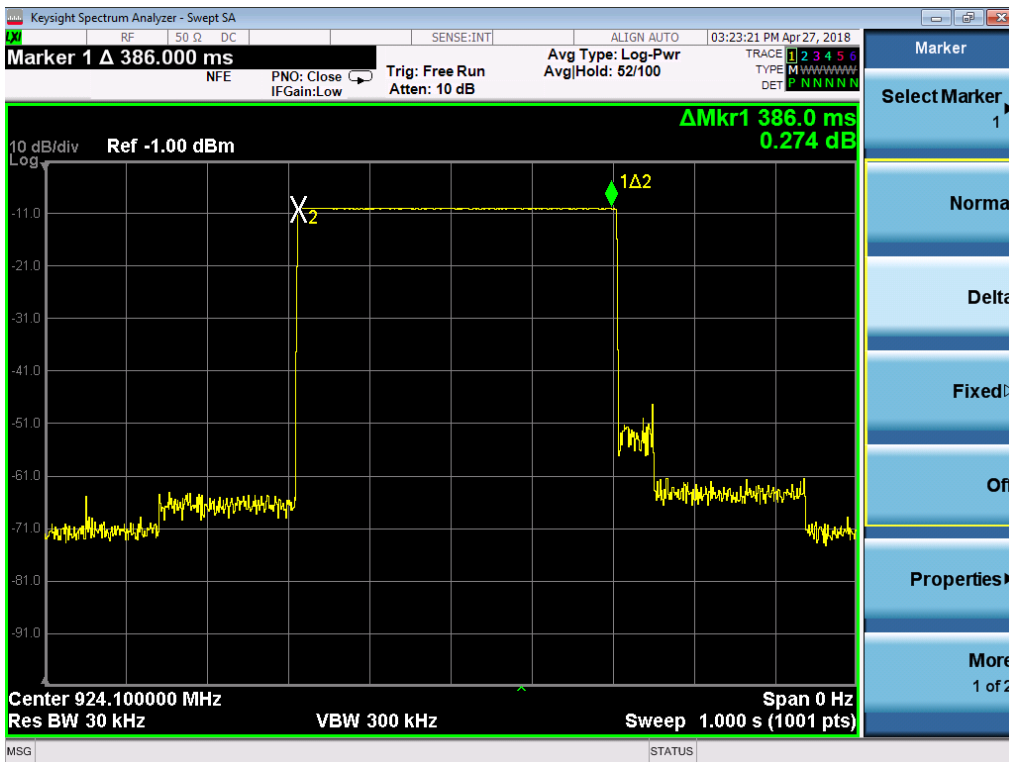
Figure 19: Bottom channel, 924.1MHz transmit time per hop
