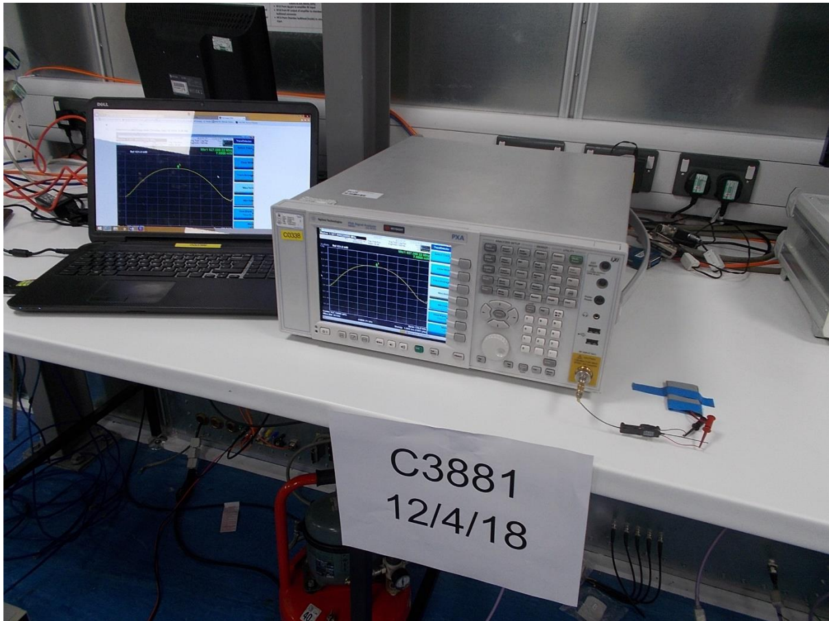
Conducted type test set up - peak conducted power
