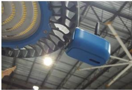
XCM attached to an EOS fixture
