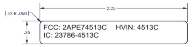
The label will be attached to the flat step feature underneath the battery holder, visible to the user whenever the batteries are changed, as shown on page 2 of 4646.OX.PDF in quadrant D2:
