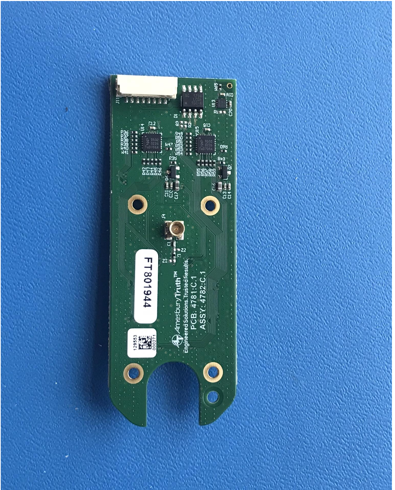
Figure 5 - Exterior Antenna/LED PCB Side 2
