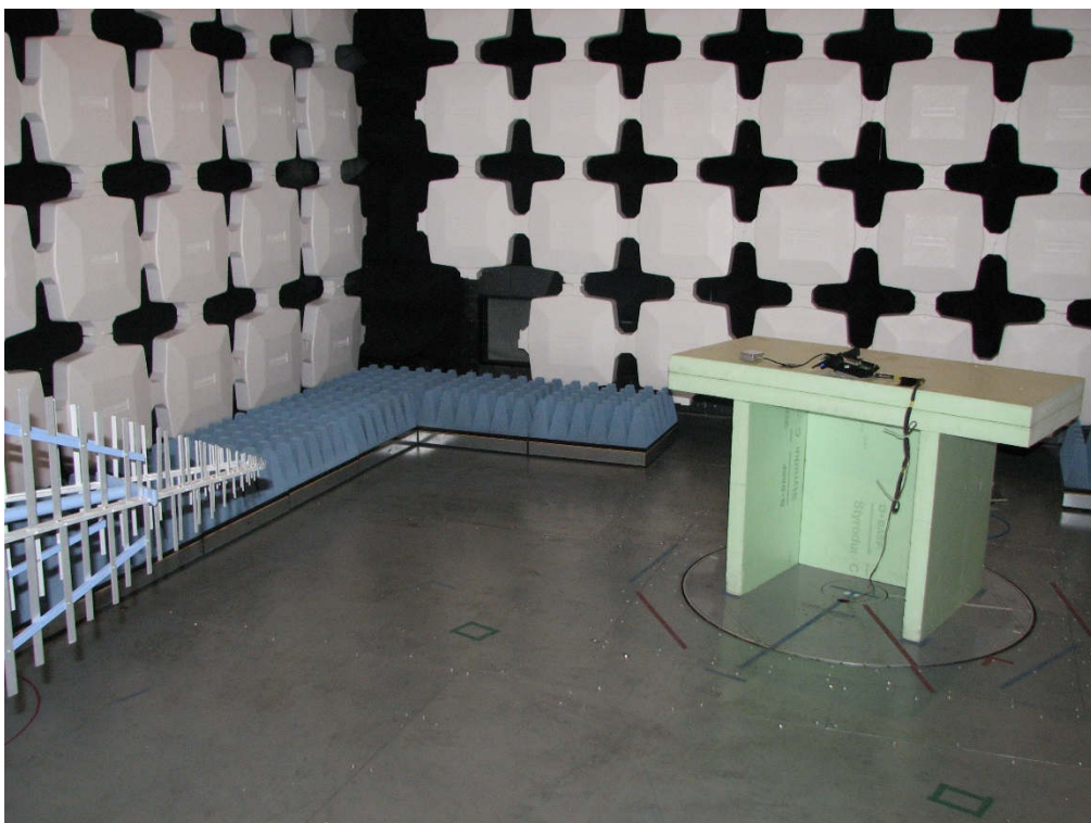
FCC Part 15C Radiated Emissions Test Setup 30-1000 MHz
